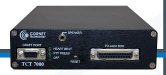
The TCT 7000 and TCT 7000J, integral members of a Cornet Switching Systems Tactical Voice Communications Subsystem (TVCS), are a SIP-based TCT-7000 operator interface unit that interfaces with a Communications Interface Panel (CIP), the operator's headset and microphone and the TVCS conference switch. It enables single or multiple-simultaneous secure/non-secure intercom, radio, or telephone calls.
