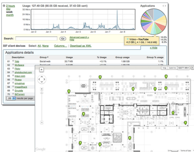
Cisco Meraki dashboard and Cloud Management - showing traffic and AP location
